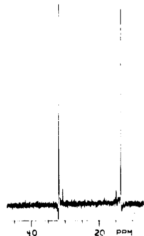
Figure 2. 13 C NMR spectrum of CH 3 and CH 2 groups of 3f (H decoupled).
